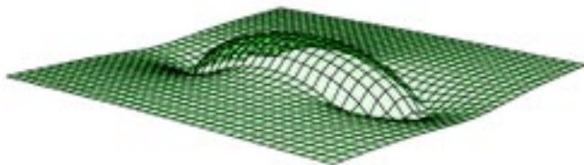
FIG. 4 (color online). Possible interfacial profile around an ellipsoidal particle. The deformations have a quadrupolar symmetry.
